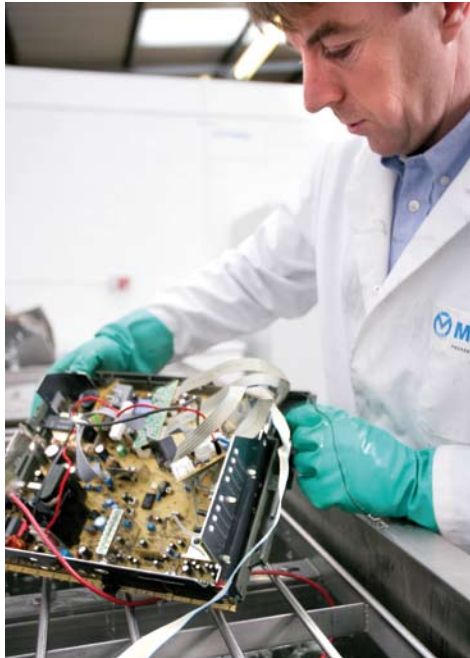
Reconditioning of a Printed Circuit Board of a TV set.
