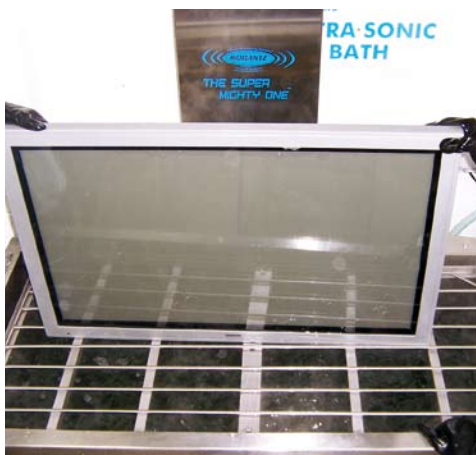
Putting a flat screen TV into the ultrasonic bath.
