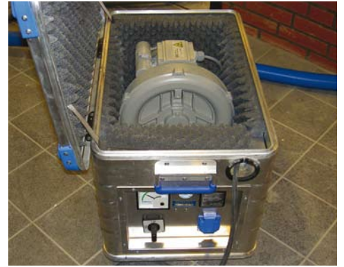
Aluminium boxed high pressure fans to reduce noise and prevent damage.
