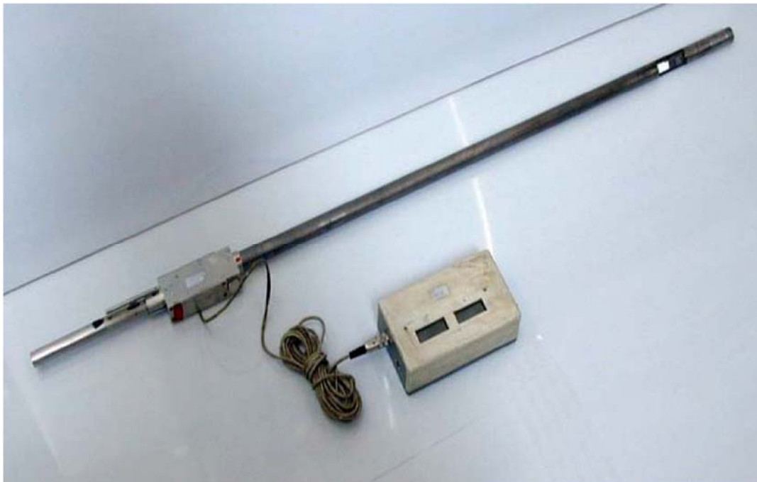
Fig. 2: Impactor Probe with time recorder (impactor with Shield Tube opened)
